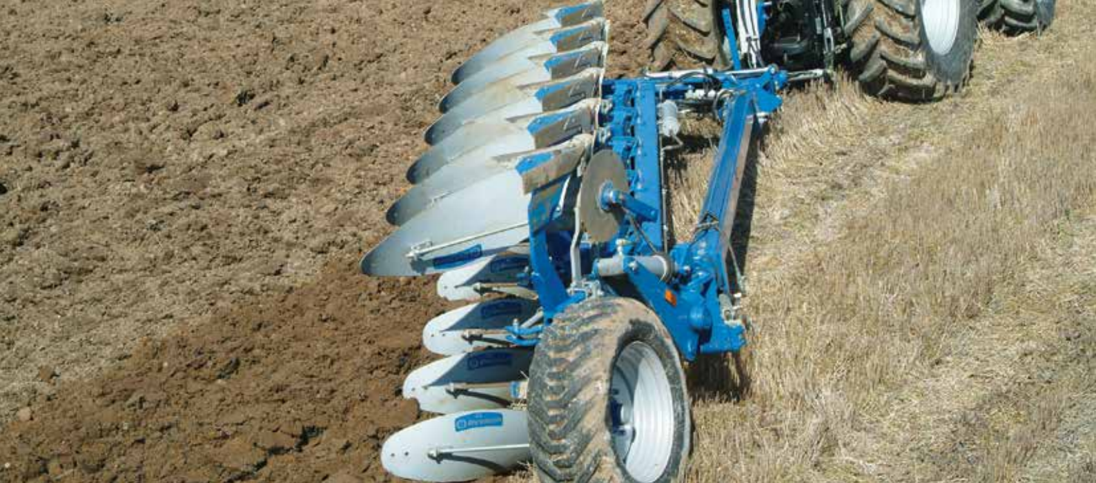
CVL 6975 H. The draw frame is placed high in order to improve clearance.
