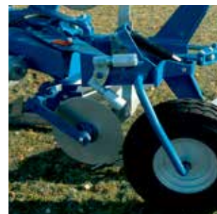
The pendulum depth wheel controls the depth of the rear part of the plough.
