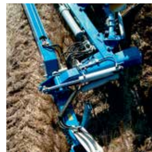
Hydraulic front furrow adjustment is standard.
