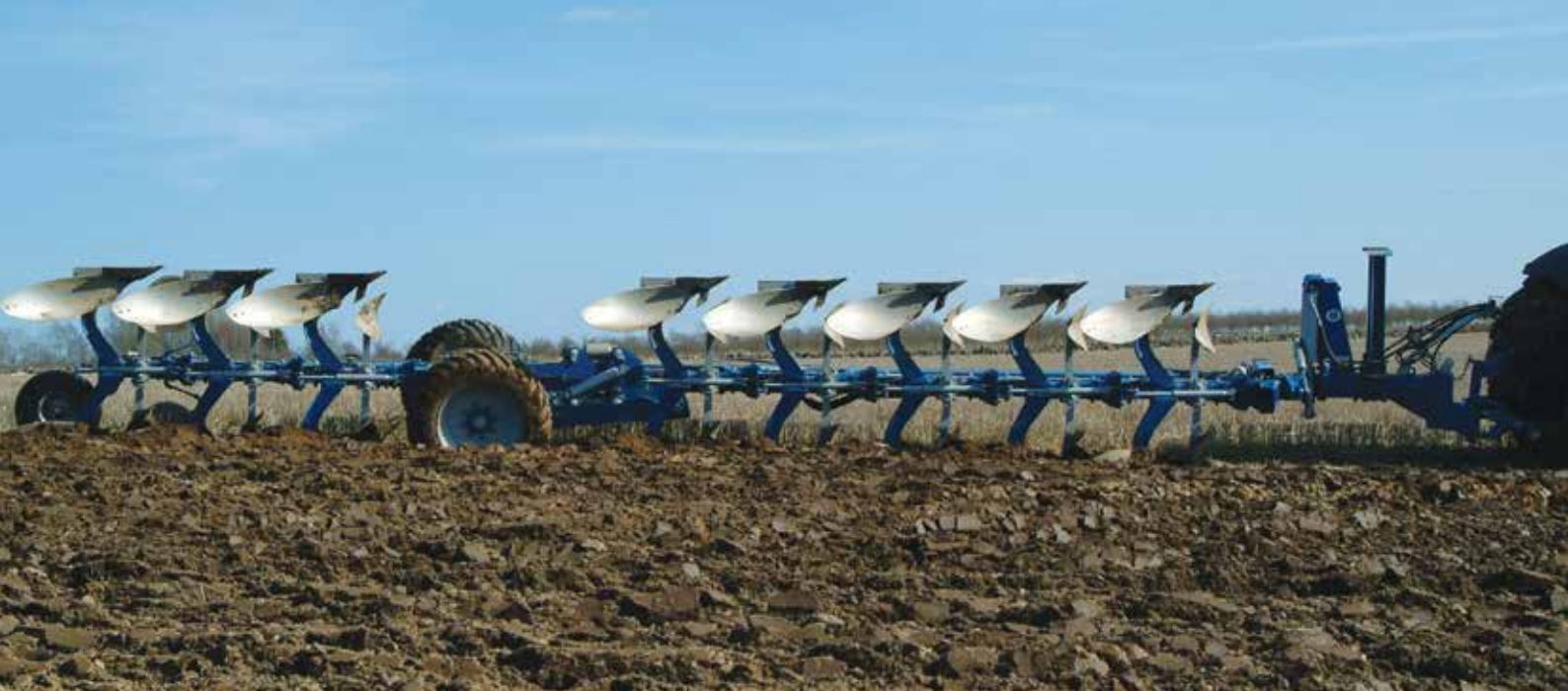
Överum DXL 81080 H. Large diameter wheels (400x26.5) mean good support and depth control also in difficult conditions.
