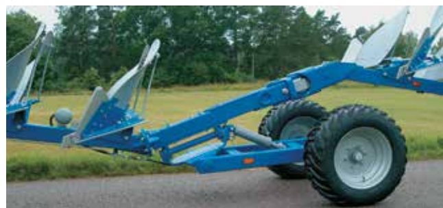
The weight distribution over the wagon makes the CXL gentle to manoeuvre. A hydraulic suspension in the lift cylinder contributes to the soft and secure transport.
