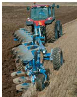
Överum DXL 81075 H. The furrow width can be set at 16, 18 or 20 inches. Optimum clearance for non-stop ploughing in heavy trash.
