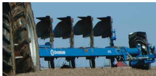
The draw frame is placed high in order to improve clearance.
