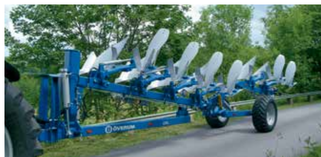
In transport position the CXL acts like a wagon with low centre of gravity.
