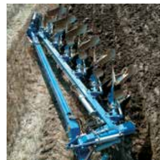
All side forces are automatically balanced out in the Överum semi-mounted plough concept.
