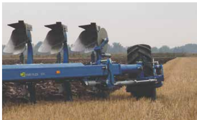
Large rear mounted depth wheel (420/70 R24) for optimum weight transfer and operation in difficult conditions. A slave cylinder secures that the wheel is aligned when the furrow width is changed.
