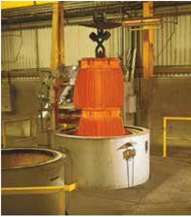
Carburizing of mouldboard blanks.
