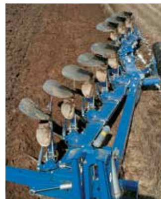
Överum DXL 81075 H. The furrow width can be set at 16, 18 or 20 inches. Optimum clearance for non-stop ploughing in heavy trash.
