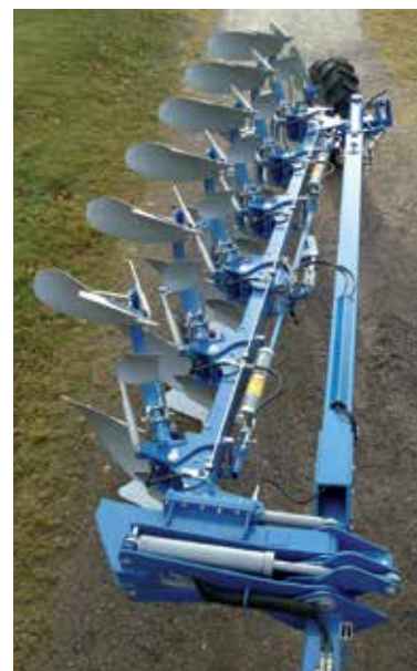
Heavy-duty beam housing design with optimum geometry for low force demand when adjusting furrow width.
