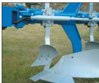
Skimmer EG. Wide shallow cut. Works well with both fin coulters and disc coulters.
