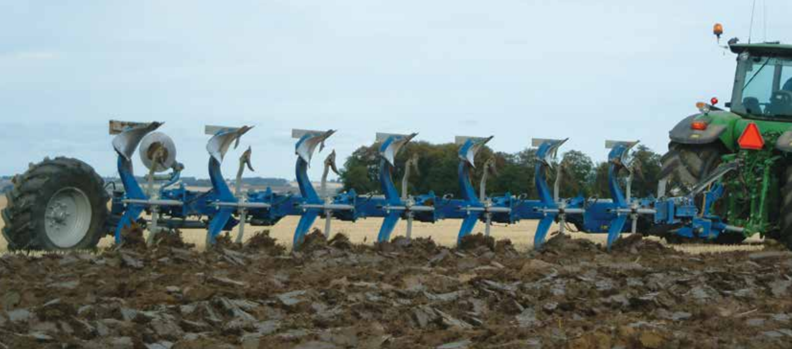
Vari Flex EVL 71080 H with hydraulic furrow width adjustment.
