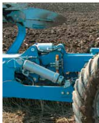
Överum DXL wagon ploughs have a hydraulically controlled joint, which is freely flexing in float position when ploughing.
