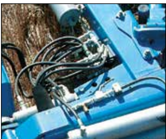
Pressure controlled diverter valve. Two double acting functions are controlled by one double acting outlet.
