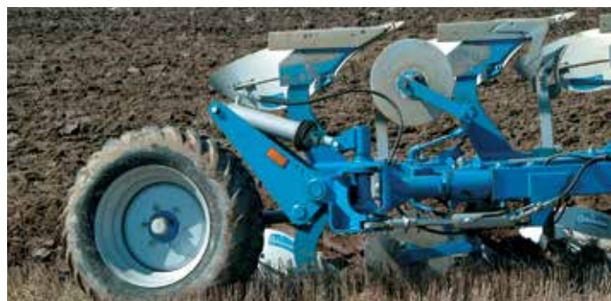
Large wheel with low rolling resistance and hydraulic steering.
