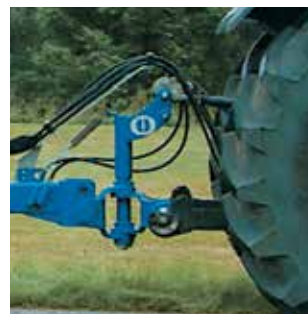
Strong hot-bent details in the draw frame.
